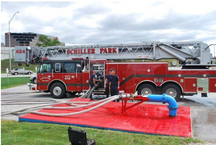
Pump Testing on Tower 5
