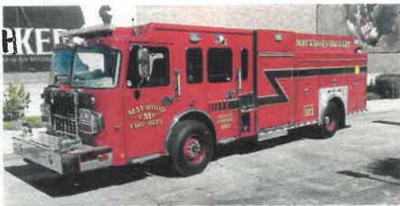
MARION —Maywood (IL) Fire Department pumper. Spartan, Metro Star cab and chassis; Cummins ISL 450-hp engine; Hale Qmax 1,500-gpm pump; 500-gallon polypropylene tank; Extend-a-Gun deck gun; enclosed pump panel. Dealer: Tony
